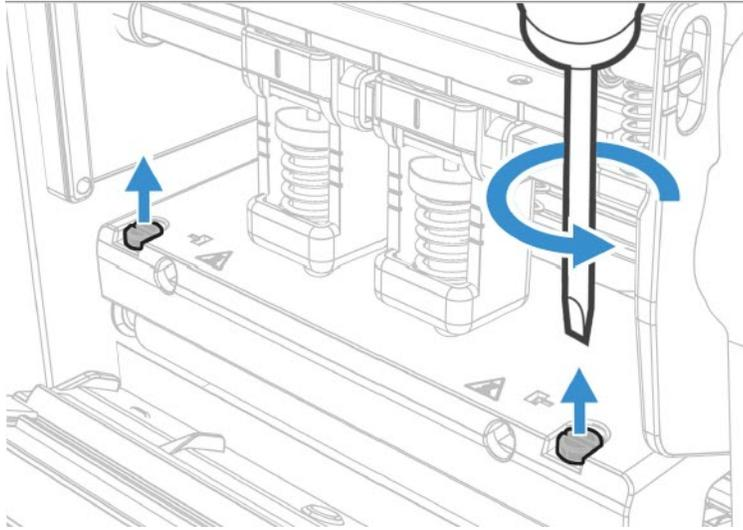
8. Turn the printhead lift lever counter clockwise and put the printhead toward you to remove.
