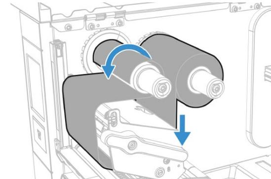
5. Turn the ribbon take-up hub counterclockwise until the ribbon becomes tight and runs wrinkle-free through the print mechanism.
