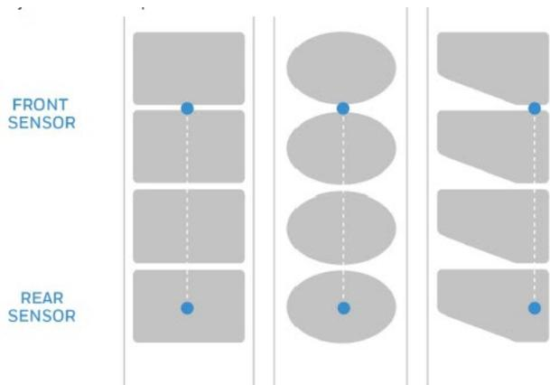
The sensor contains a blue LED that is strong enough to see through media. You can use the blue LED to help determine the proper location for the sensor.
