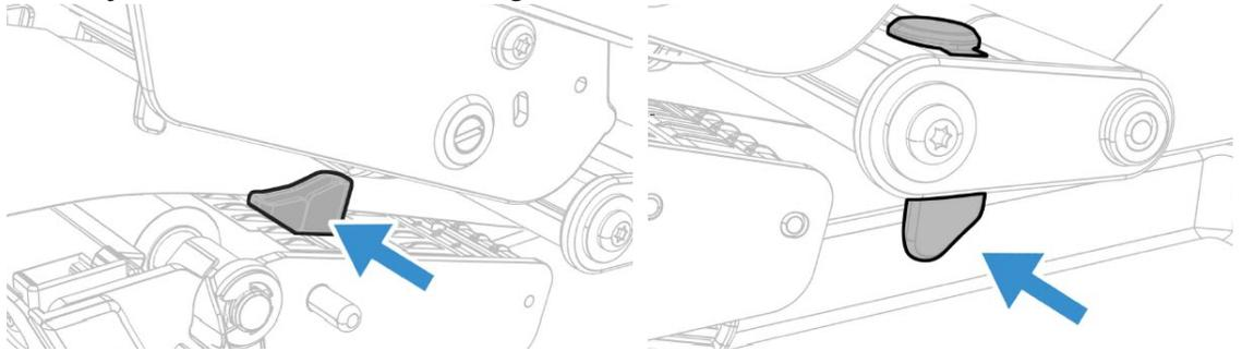
6. Lift the cutter plate into place, lower the front arm, turn the printhead lift lever clockwise to close the printhead and click into place.
