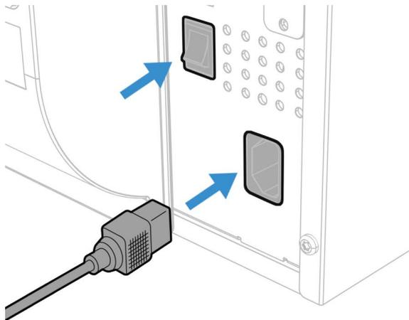
2. Press the power switch to turn on the printer.
