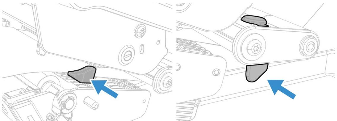
**Note:** There is a media guide that is located near the printhead. It is recommended to adjust the media guide all the way to the right in order to insert the media. If not, it can be difficult to load the media.
