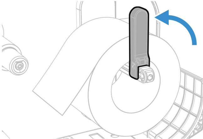
5. Turn the printhead lift lever counterclockwise to raise the printhead and lift the front arm.
