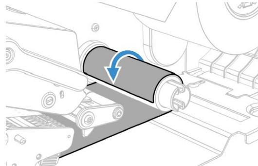
3. Lift the rewriter batch plate into place, lower the front arm, turn the printhead lift lever clockwise to close the printhead and click into place.
