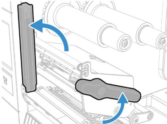
6. Route the media through the print mechanism, through the front arm.
