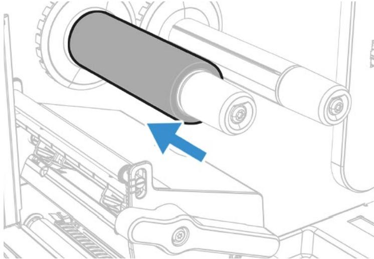
**Note:** For ribbon that has the ink wound out, place the ribbon on the ribbon rewind hub with the ribbon wound clockwise. For ribbon that has the ink wound in, place the ribbon on the ribbon rewind hub with the ribbon wound counterclockwise.
