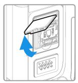
8. Press down gently and slide the card holder away from the open access door. Lift the edge of the holder up.
