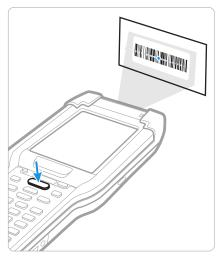
4. Release the Scan button when the computer beeps, and the Scan Status LED briefly turns on. The barcode information is entered into the application in use.
